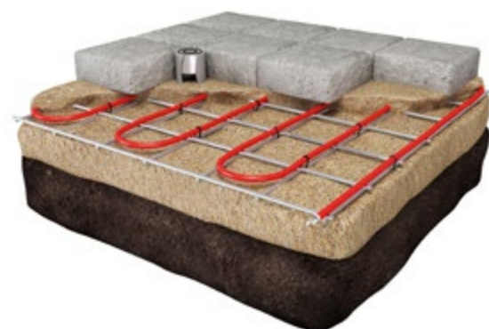
Installation in sand bed under paving stones
