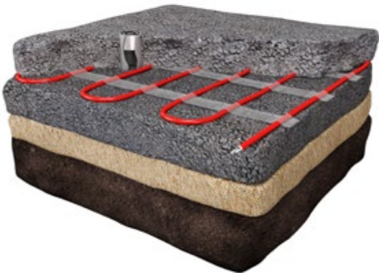
Installation in unrolled asphalt
