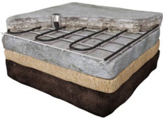
Installation in concrete
