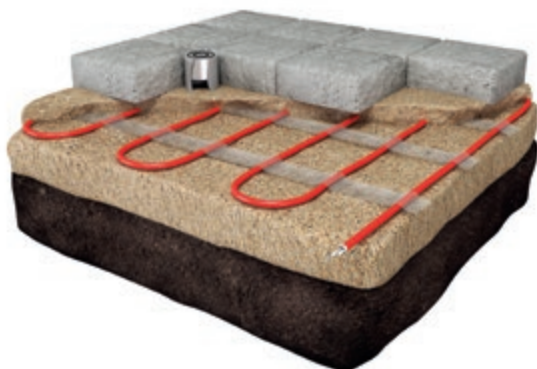
Installation under paving stones
