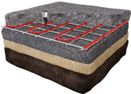
Installation in unrolled asphalt
